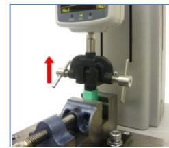
USB connector extracting/inserting force test
